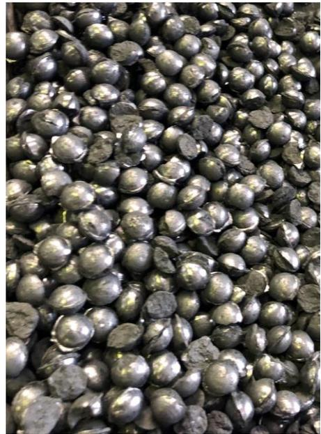
Pelletised carbon pellets – source Company
